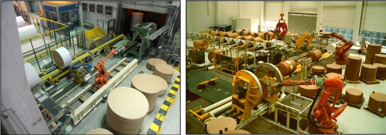
Figure 1. Paper roll packing methods can be divided to two main categories: stretch (on the left) and kraft wrapping (on the right).
