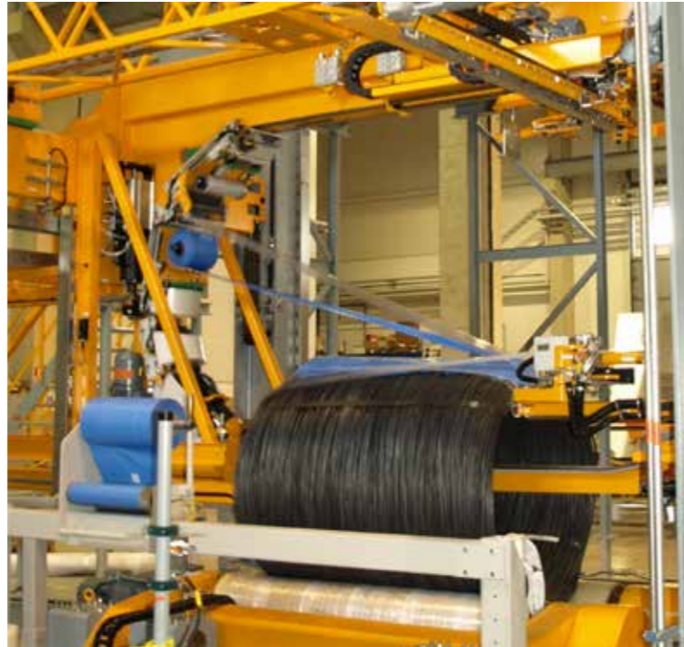
TEW (through eye wrapping) with fabric and film.
