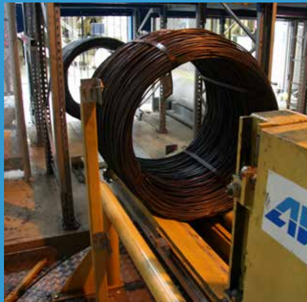
TransCoil channel vehicle can handle multiple coils simultaneously.
