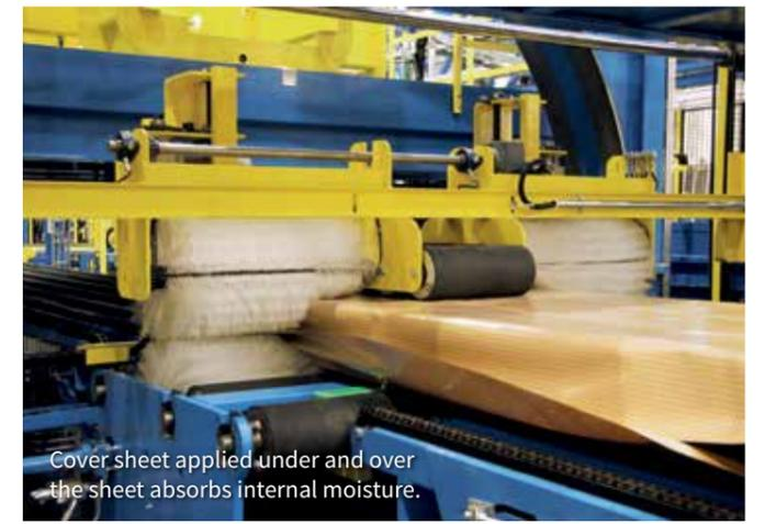
Cover sheet applied under and over the sheet absorbs internal moisture.
